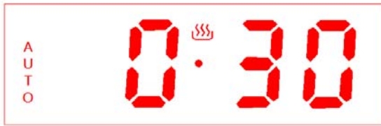
Pic 24 Cooking time well set diagram
