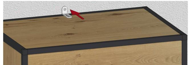
Mounting the tilt protection for highboards
