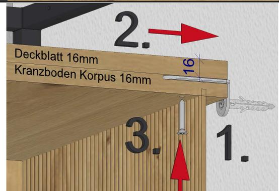
**Use of the tilt protection is absolutely necessary!**
