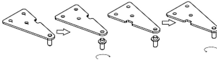
7. Fit in the top door. Move the top hinge to the left side. Before you tighten the top hinge, ensure proper horizontal and vertical position of the top door so the door seals will close properly.
