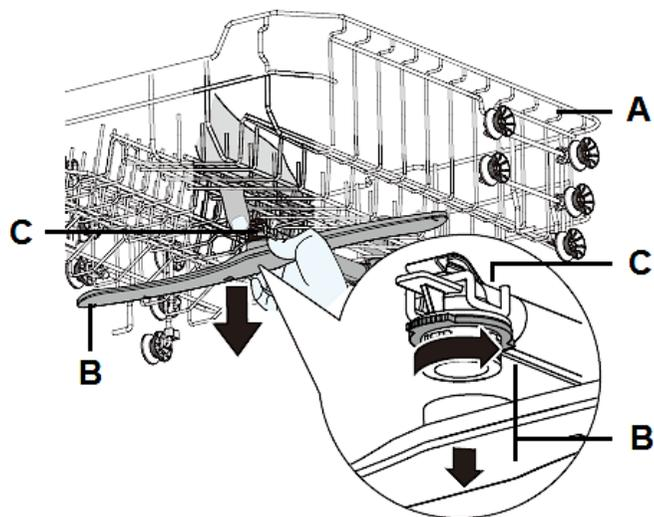
(2) To remove the lower spray arm (D), pull it out upwards (s. fig. below, arrow).
