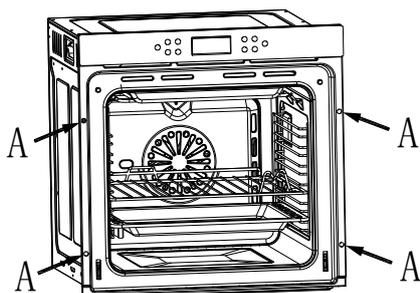
Ensure that the oven has been securely fixed into the housing unit. The fixing of the oven into the housing is made by using four screws. These should be screwed through the oven cabinet and into the housing unit.
