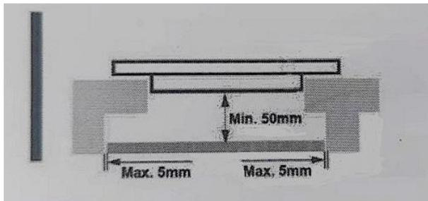
There are ventilation holes around outside of the hob. YOU MUST ensure these holes are not blocked by the worktop when you put the hob into position. Be aware that the glue that join the plastic or wooden material to the furniture, has to resist to temperature not below 150°C, to avoid the unstuck of the paneling.
