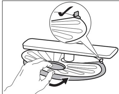
7. Reassemble the filters (B) and (C).
