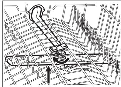
3. Wash the spray arm under running water. Use a thin pointed tool, e.g. a toothpick, to remove particles of soil from the holes.
