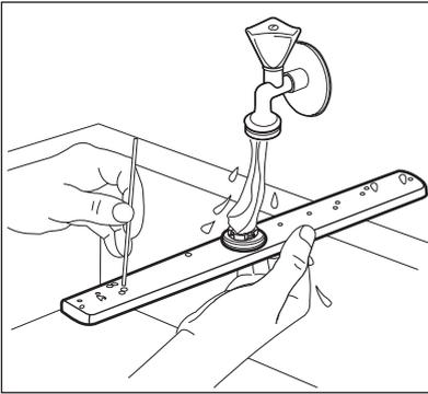
4. To install the spray arm back, press the spray arm upwards and
