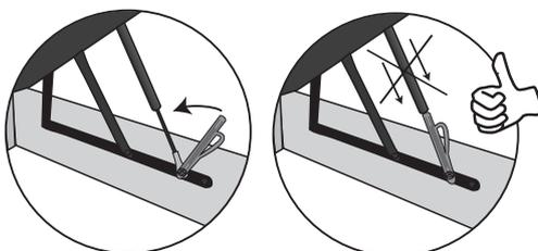
Put the plastic stopper to the gas spring so that the bed box can't close
