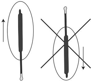
The piston of the gaspring must be at the top
