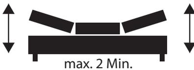
Do not use the motor lifting function for longer than 2 minutes at a time
