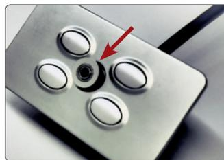
sit in the chair during charging or connect the cable while you are sitting. The cable could be pulled out, damaging the charging socket.
