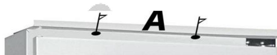
Fixing points to fix the appliance with the assembled components A+B and the supplied woodscrews in the cabinet.
